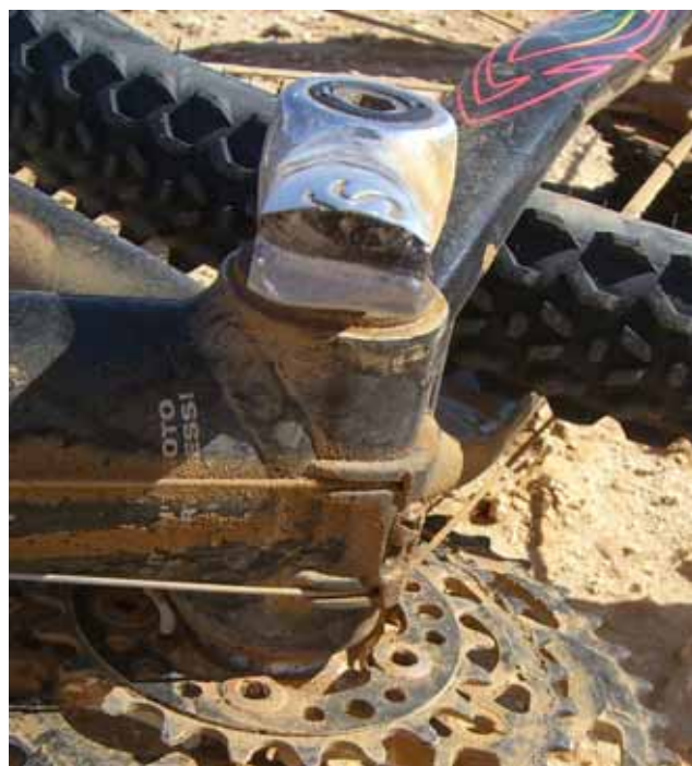
A broken crank.. very rare but you never know. Breakages on the race include seat posts, handlebars, frames, derailleurs, chains.
